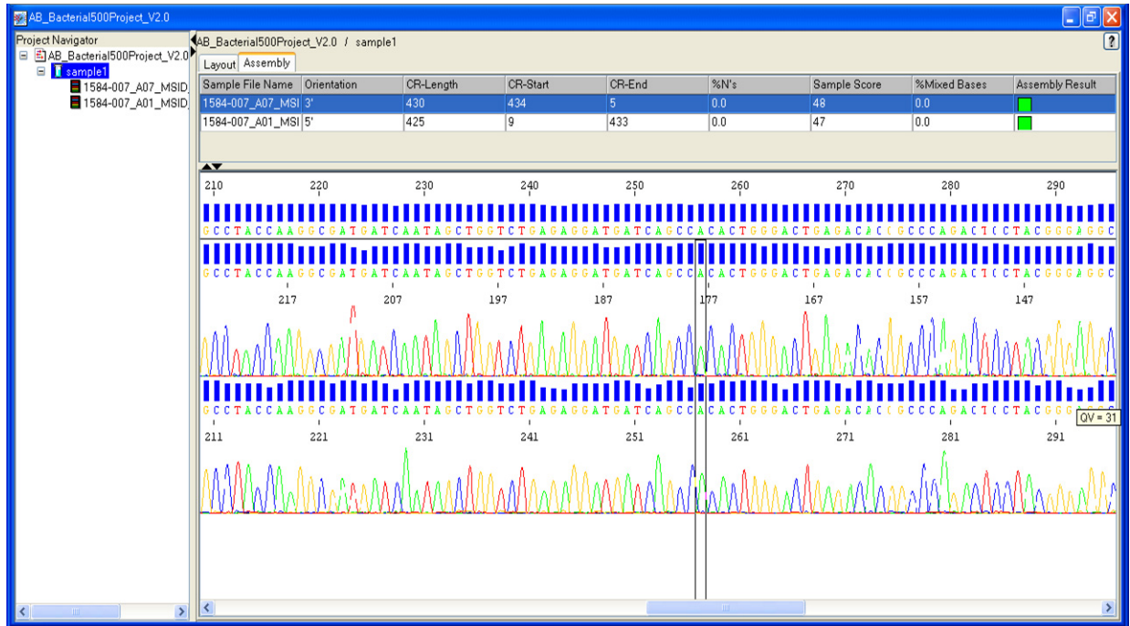
Figure 24 MicroSeq® ID Analysis Software, showing the alignment of the forward and reverse sequences of a sample (with electropherograms) to the consensus sequence generated by the software (at the top). The consensus sequence is compared to the validated library.
